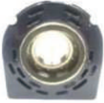
myTVS P.No:RCJ9092 CENTRE BEARING ASSY. W/BEARING 6211(2RS) 2518 N/M (CUT TYPE)
