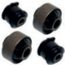
myTVS P.No:UHC2 FRONT LOWER ARM BUSH 2 PCS (CITY TYPE 3)
