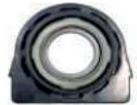
myTVS P.No:RCJ9029 CENTRE BEARING ASSY.(2 SPOKES) W/BRG. 6211 (68 MM-CUP)
