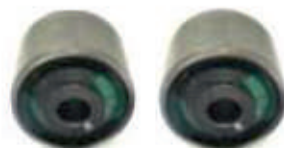
myTVS P.No:UMS35A LOWER LINK CHASSIS BUSH (14 I.D.) .. 2 PCS SCORPIO TURBO CRDE
