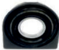
myTVS P.No:RCJ9097 CENTRE BEARING ASSY. TATA2518/ 3118 (BUSH) W/ BRG. 6013 (RSB TYPE) (2 RS)
